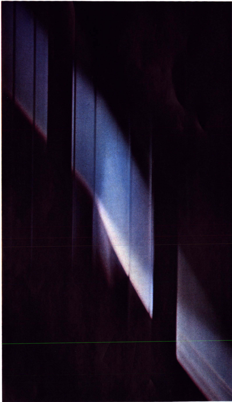
Fig. 8. Streak picture. p_0 = 0.5 torr, B_0 = 6.8 kG.
